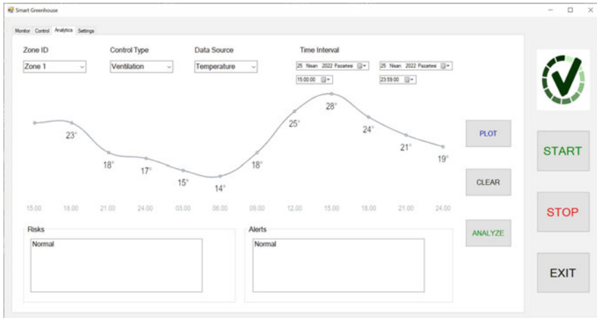
Fig. 9 Data analytics function of developed digital twin software
