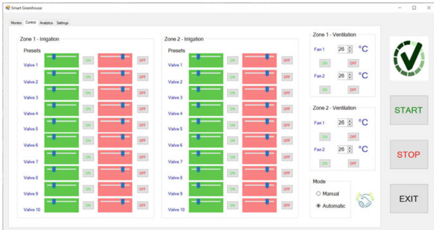
Fig. 8 Control function of developed digital twin software
