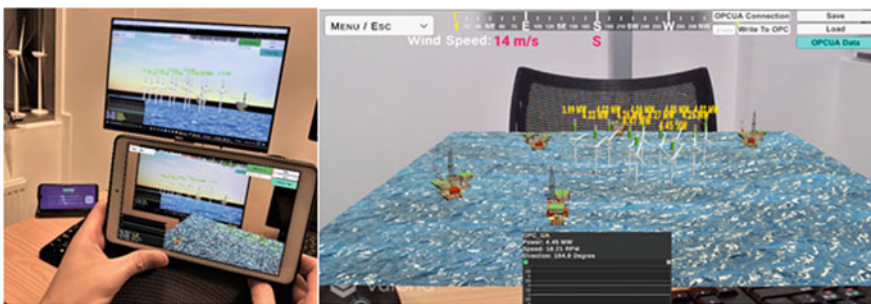
Fig. 6 Interactive digital twin platform based on augmented reality
