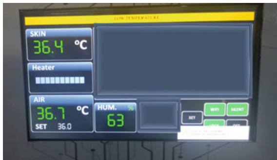
Fig. 3 Temperature on a baby incubator display. On the display there are temperature settings, display room temperature, skin temperature, humidity and display heater performance
