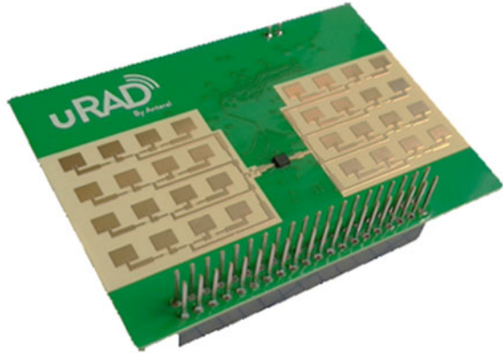
Fig. 1 URAD radar as a tool for detecting the movement of SIBI letters and numbers
