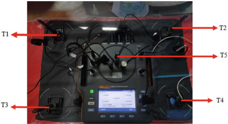
Fig. 2 Temperature data collection utilizing the Fluke INCU 2 type Incu Analyzer with temperature parameters T1, T2, T3, T4, and T5
