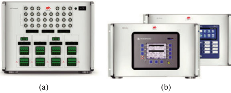
Fig. 1.15 HIL interfaces: a HIL connect; b Packaged interface with HIL compatible controllers
