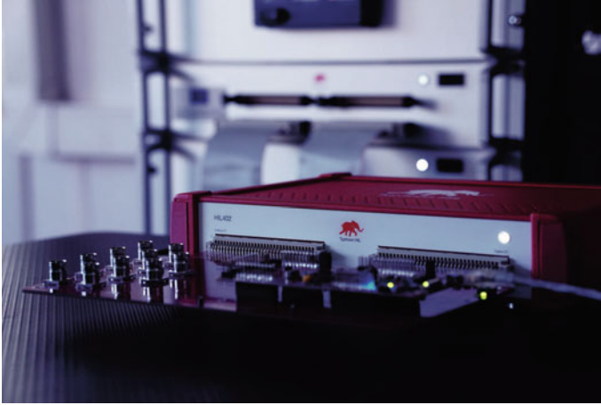
Fig. 1.22 Example of C-HIL setup with a Typhoon HIL402 real-time simulator, TI LaunchPAD LAUNCHXL-F28379D, and a dedicated interface board
