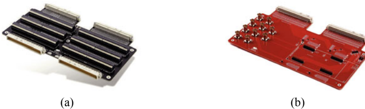
Fig. 1.14 HIL interfaces: a HIL breakout board; b HIL TI launchpad interface
