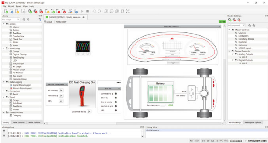
Fig. 7.3 Typhoon HIL SCADA
