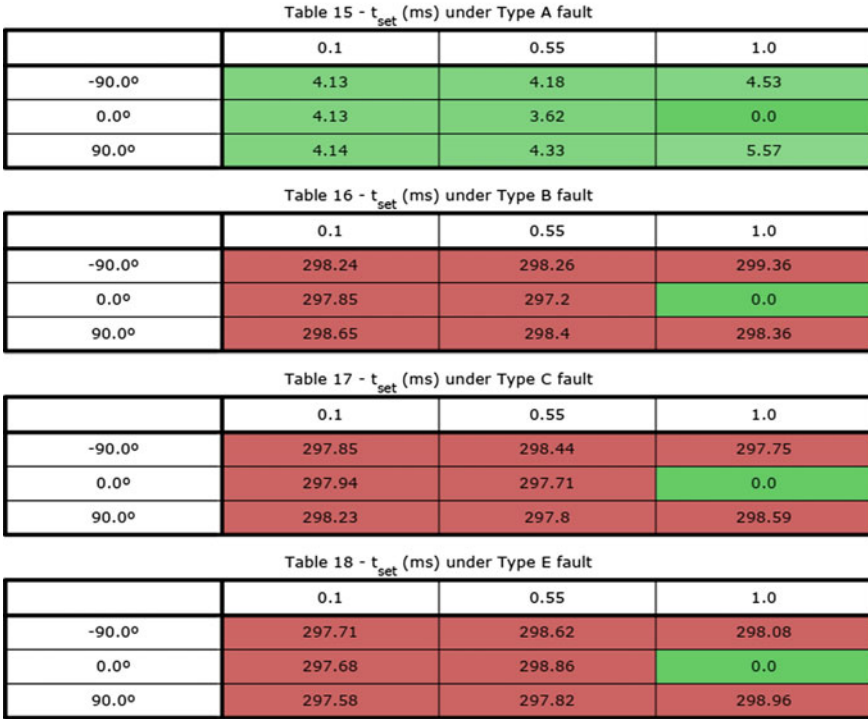
Fig. 4.5 SVM 2 PC: colour-graded table showing the settling time (performance index) for different grid faults
