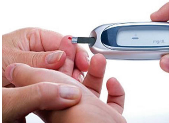
Fig. 17.1 Invasive glucometer showing blood collected in the test strip after painful prick
