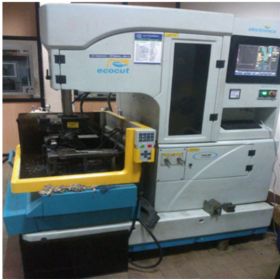
Fig. 1 ECOCUT® CNC wire-EDM machine set-up
