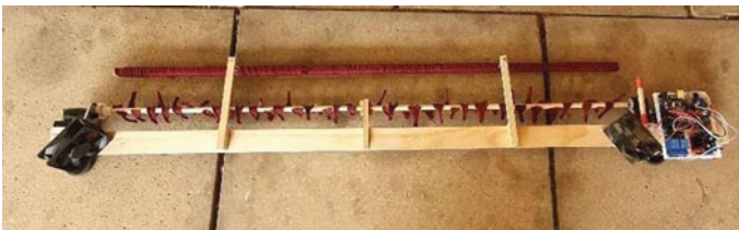
Fig. 14.13 An Arduino based solar panel cleaning system
