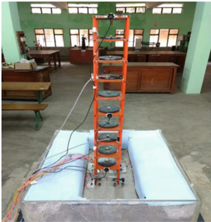
(b) Flexible Base Structure- Pile group
