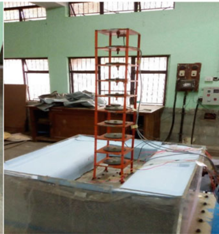
(c) Flexible Base Structure- Piled Raft
