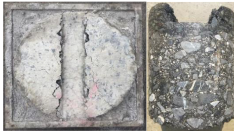
Fig. 7. Loaded specifications and drilled core sample
