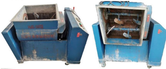
Fig. 2. HJS-60 horizontal double-axis forced mixer.
