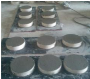
Fig. 2. Forming Method of Salt Frozen Specimens
