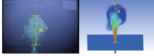
Fig. 6. Actual height of drilling fluid return and simulated height
