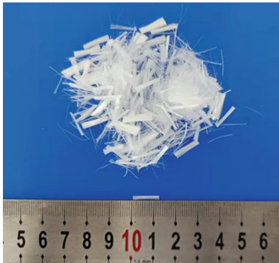
Fig. 3.6 Appearance of PVA fiber. Reproduced from Development and design of ultra-high ductile magnesium phosphate cement-based composite using fly ash and silica fume by Hu Feng with permission from Elsevier
