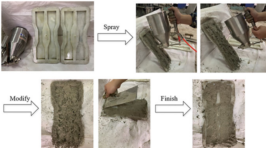
Fig. 6.6 Experimental process. Reproduced from Development of sprayable ultra-high ductility magnesium phosphate cement-based composites based on the rheological properties by Hu Feng with permission from Elsevier
