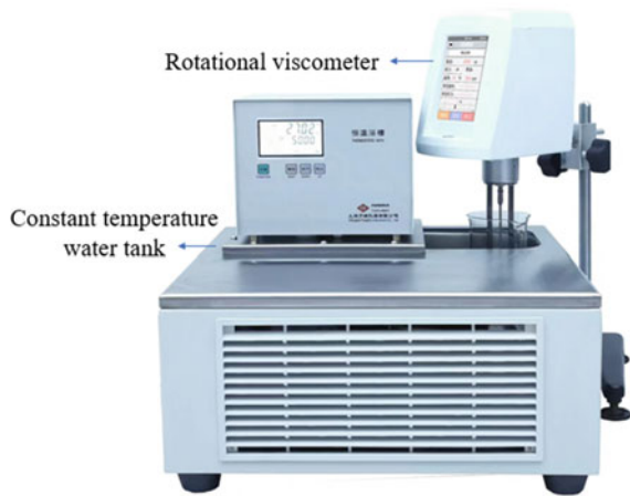
Fig. 6.8 RVDV-1T rotational viscometer and constant temperature water tank. Reproduced from Development of sprayable ultra-high ductility magnesium phosphate cement-based composites based on the rheological properties by Hu Feng with permission from Elsevier
