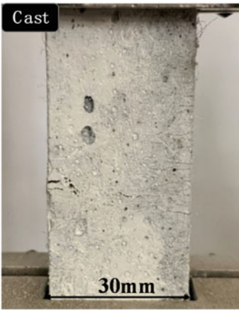
(c) Cracking diagrams of UHDMC with V_f of 2.0%
