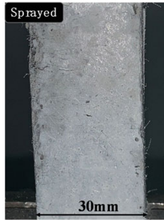
(c) Cracking diagrams of UHDMC with V_f of 2.0%
