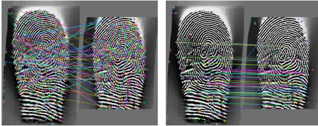
Fig. 3. False Minutiae Removal processing. It is apparent from the comparison images that False Minutiae Removal has a significant impact on the accuracy of fingerprint alignment. The image on the left shows a significant amount of interference in the form of non-discriminative keypoints, while the image on the right demonstrates the effects of removing these undesirable keypoints.
