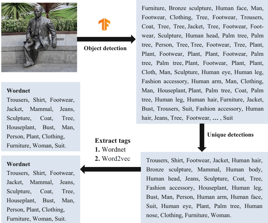
Fig. 2. Object detection and tags grouping
