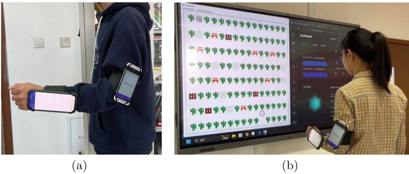
Fig. 7. System test (As an illustration, we implement KylinArm on two smartphones. However, the use of two smartphones is not necessarily required, one of them can be replaced by a smartwatch or other IMU-equipped device.): (a) IMUs Position (b) Interact with the game through arm gestures
