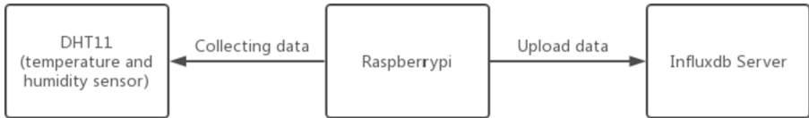
Fig. 9. Temperature data acquisition.
