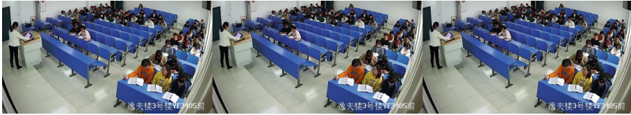
Fig. 5. The prediction effect of different detection head sizes. The left picture is the prediction effect after 200 rounds of model training corresponding to 40 \times 40 and 80 \times 80 sized detection heads, the middle picture is the prediction effect after 200 rounds of model training corresponding to 20 \times 20 and 40 \times 40 sized detection heads. The figure on the right is the prediction effect after 200 rounds of model training corresponding to 40 \times 40 and 80 \times 80 sized detection heads. These three models are identical except for the different detection head sizes.
