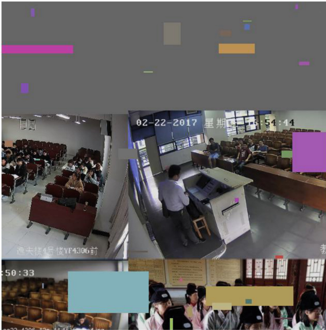
Fig. 4. Mosaic and Cutout. Using the Mosaic data enhancement method, four plots are randomly cropped and put together into a single plot, and the different colored and sized squares in the plot are the effect of Cutout data enhancement.
