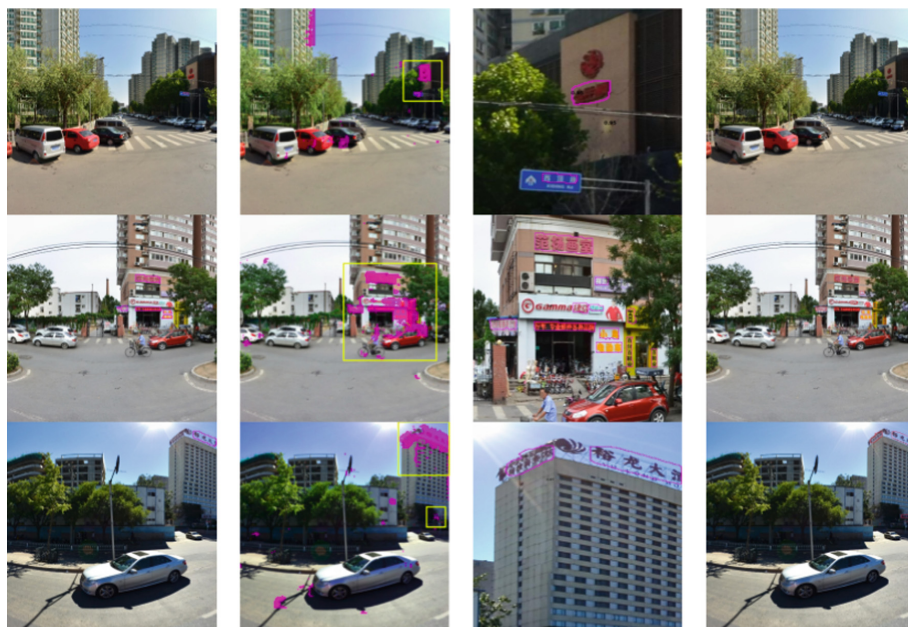
Fig. 7. Inference pipeline in TextFocus. All results are processed on the Large CTW dataset [2]. Focus Pixels masked as pink, interesting region chips are shown in yellow in the second and fourth rows. Text instances detected in each chip are shown in purple in the first and third rows, final detection results are shown in red in last row. As can be seen, high resolution image samples contain small text instances and some of them can be detected in the higher scale.
