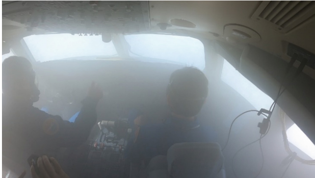
Fig. 4. At 12:16:20 An overall View of the Cockpit when Smoke Evacuation Test Stops
