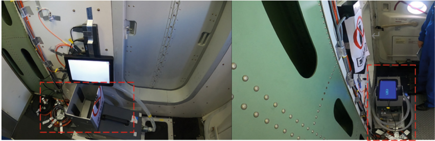
Fig. 1. Smoke Generator Installation
