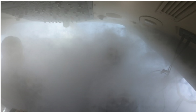
Fig. 3. At 12:15:52 An overall View of the Cockpit When Smoke Generation Stops
