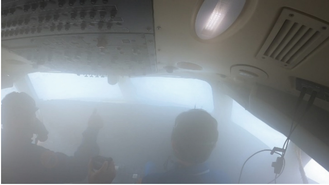
Fig. 12. At 12:29:24 Overall View of the Cockpit when Smoke Evacuation Test Stops
