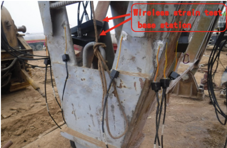
Fig. 8. Field test diagram 1 of wireless strain test system
