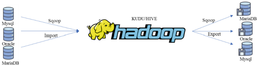
Fig. 4. The principle of using Sqoop technology to access data to Hadoop.
