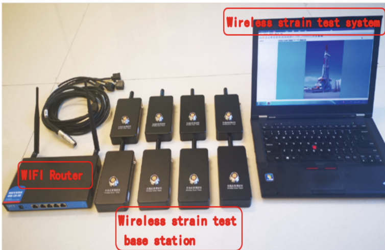
Fig. 2. Physical diagram of wireless strain testing system
