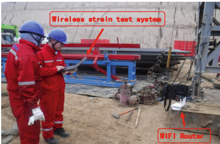
Fig. 9. Field test diagram 2 of wireless strain test system
