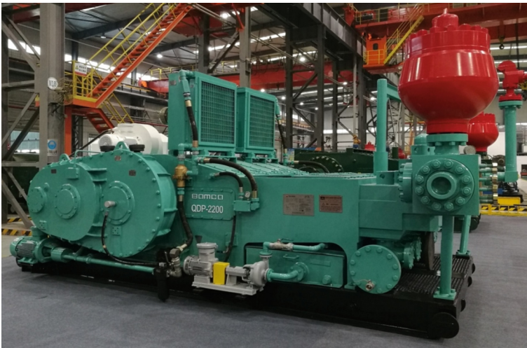
Fig. 1. Overall structure diagram of QDP- 2200 five-cylinder pump
