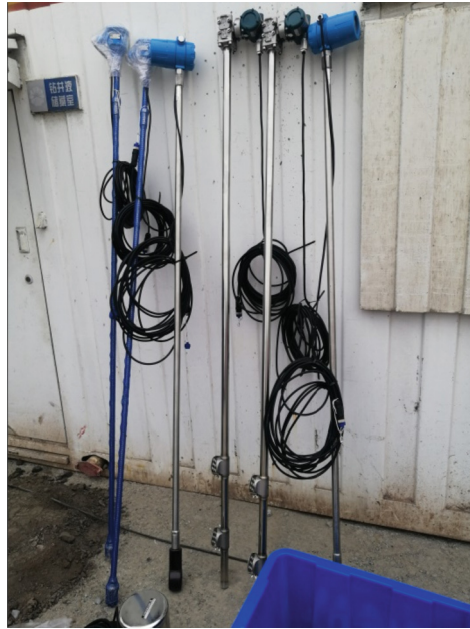
Fig. 1. Partial sensors of comprehensive mud logging instrument
