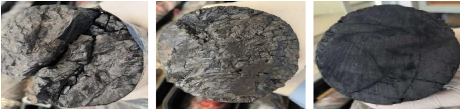
Fig. 1. Display of micro cracks and cleats in Taiyuan Formation coal seams
