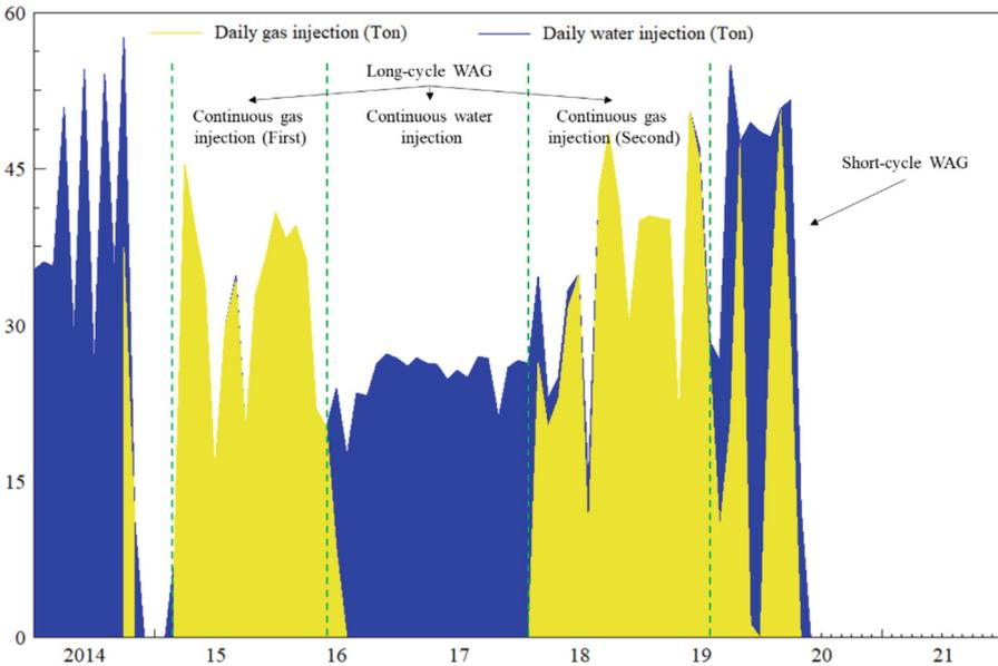
Fig. 3. Analysis of WAG phase in detail
