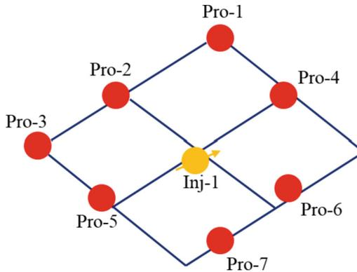
**Fig. 1.** A diamond-shaped inverse nine-point well pattern in the well group
