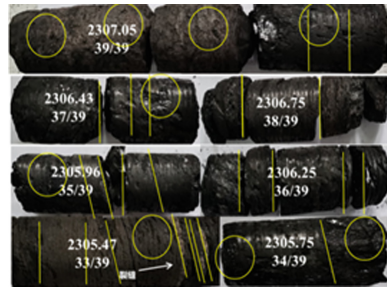
Fig. 11. Fracture distribution of core sample
