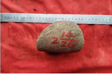
Fig. 3. Fine sandstone (ZZ1-2well, 2363.24–2363.40 m)
