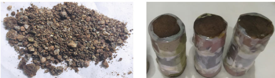
Fig. 8. Unconsolidated core samples and artificial core models
