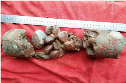
Fig. 1. Glutenite (ZZ1-2well, 2363.88–2364.19 m)
