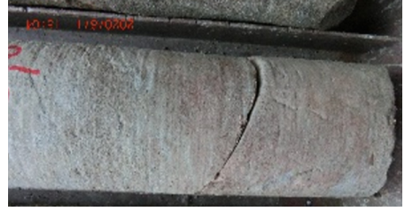
Fig. 4. Siltstone (ZZ1-2well, 2227.38–2227.53 m)
