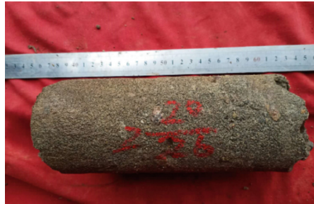
Fig. 2. Medium sandstone (ZZ1-2well, 2364.33–2364.58 m)
