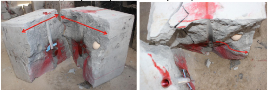
(c) Sample D3: Hydraulic fracture turn when encountering the hole
