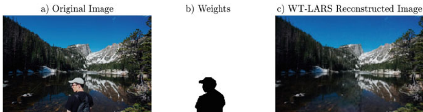
Fig. 3.3 a Original image with a person b weights image with zero weights for the person c WT-LARS reconstructed image (Person Removed)
