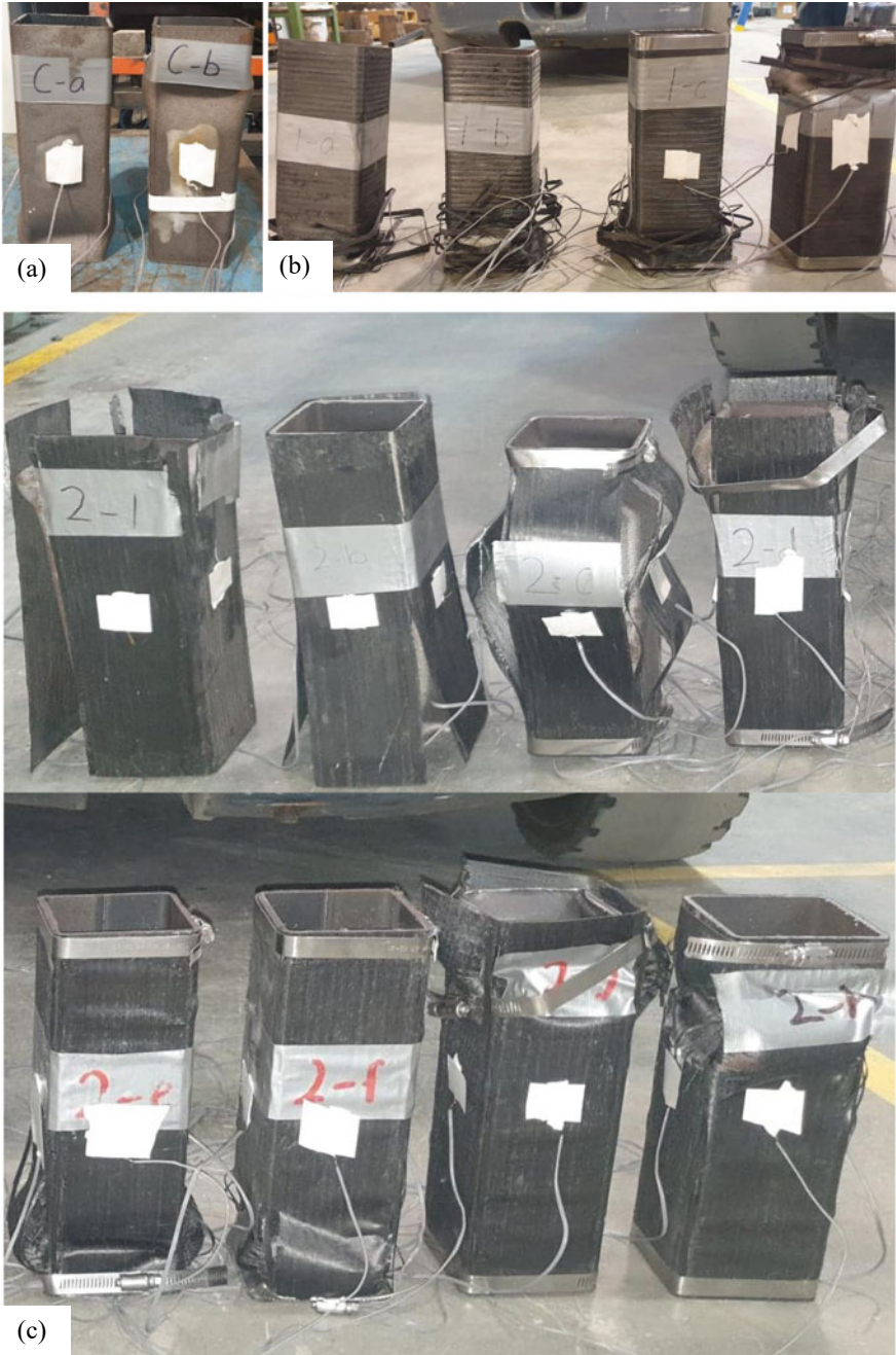
Fig. 26 Failure mode of: a control columns, b transverse CFRP columns with and without steel hose clamps, and c longitudinal CFRP columns with and without steel hose clamps
