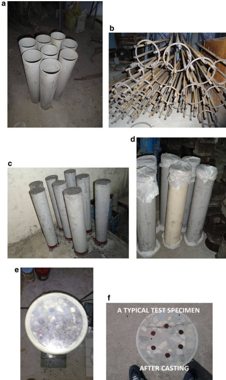
Fig. 1 a Unfilled UPVC pipes. b Reinforcement for UPVC columns. c UPVC pipes filled with concrete. d UPVC pipe columns sealed against water loss. e Epoxy capping on the test. f Cross-section of prepared specimen
