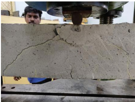
Fig. 10 Concrete Crushing in control beam
