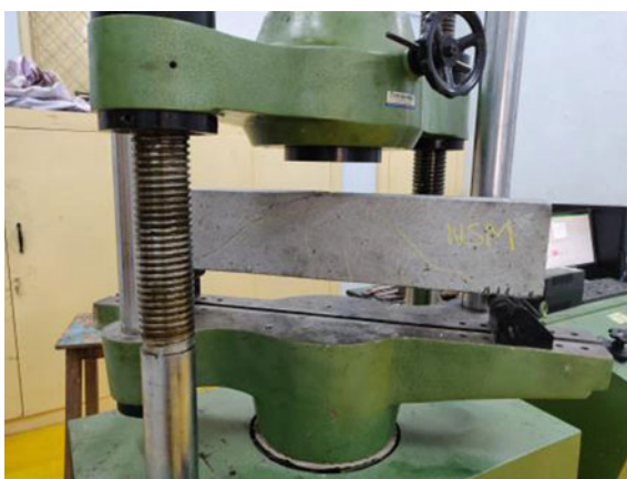
Fig. 11 Cracking in NSM specimen
