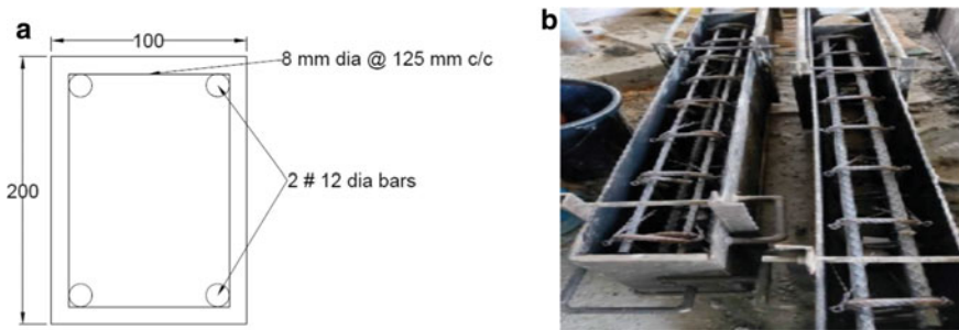
Fig. 1 a Cross-section details. b Reinforcement details
