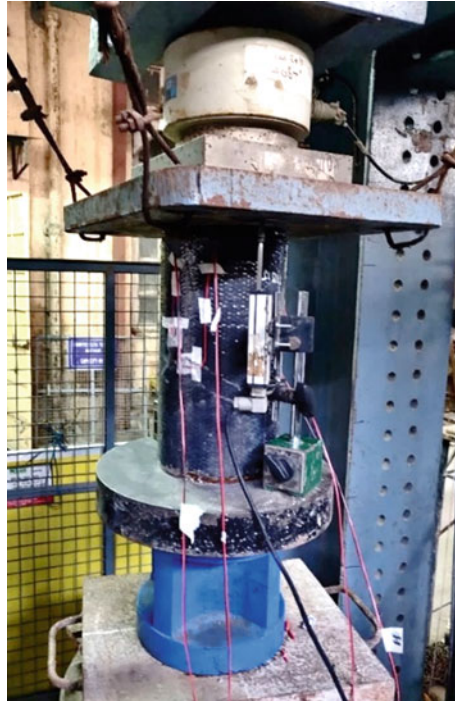
Fig. 11 Experimental setup for testing the FRP wrapped specimens in axial compression. Strain gauges attached
