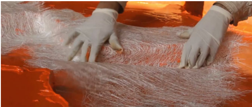
Fig. 29 GFRP fibres used to produce custom light weight formwork based on CNC cuts
