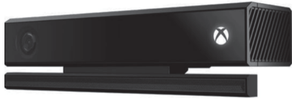
Fig. 3.35 Kinect II with its TOF technology
