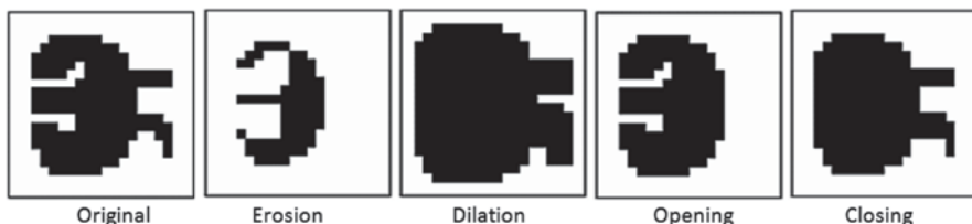
Fig. 3.18 Comparison of different processes of fundamental morphological filtering with an illustration of their use on a binary image, courtesy of [55]
