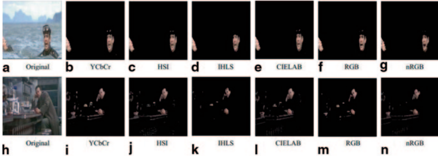
Fig. 3.4 Example results of skin detection using static skin filters in different color spaces. Black shows non-skin. (Courtesy of [39])
