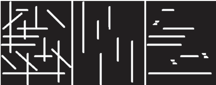
Fig. 3.16 Opening the image on the left with a 3 \times 9 structuring element (result shown in the middle ), opening with 9 \times 3 structuring element ( right )
