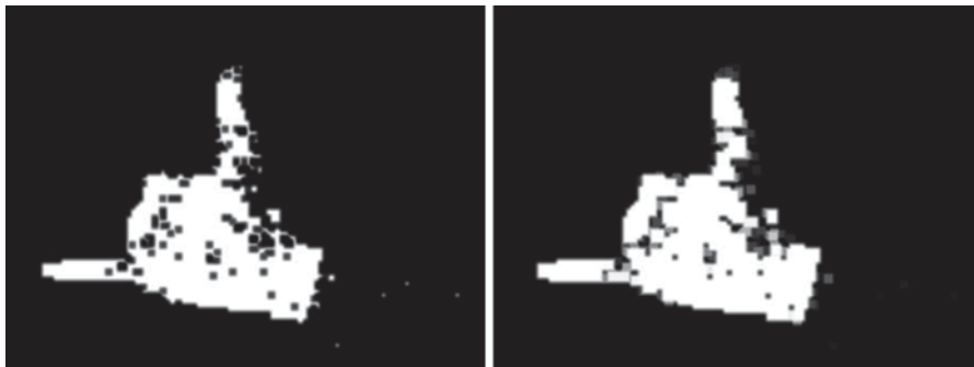
Fig. 3.12 Dilation of an eroded image with a structural element of size 5 \times 5 ( left ) and 7 \times 7 ( right )
