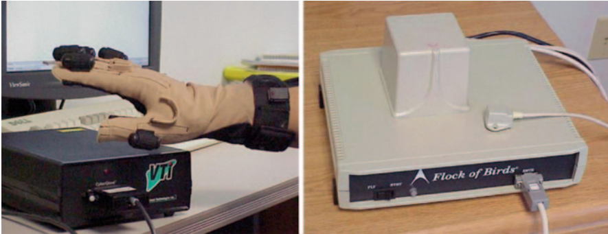
Fig. 6.19 Cyberglove™ and Flock of Birds® 3-D motion tracker. (Courtesy of [71])
