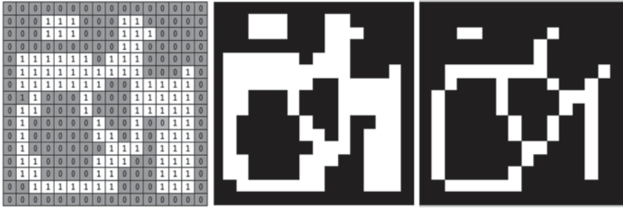
Fig. 3.22 Thinning of a binary image. The image on the left shows the pixel arrangement where some regions are 4 pixels wide. The sections with 1 pixel width remain unchanged
