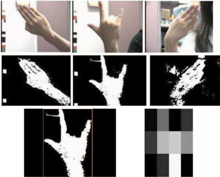
Fig. 4.13 Hand gestures in HSV space ( top row ), their binary representation after skin segmentation ( middle row ) and a gesture and its gray scale block feature vector ( bottom row ). (Courtesy of [20])
