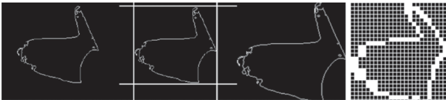
Fig. 4.11 Normalization operation and features calculation via dividing the gesture edge map with remapping. (Courtesy of [19])
