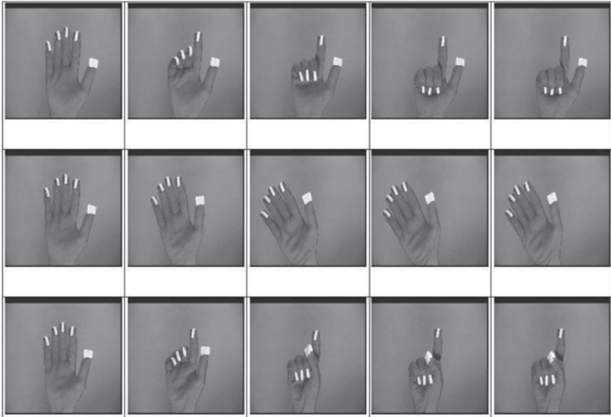
Fig. 2.10 Gesture tracking using coloured finger tips of the glove. (Courtesy of Davies et al. [15])
