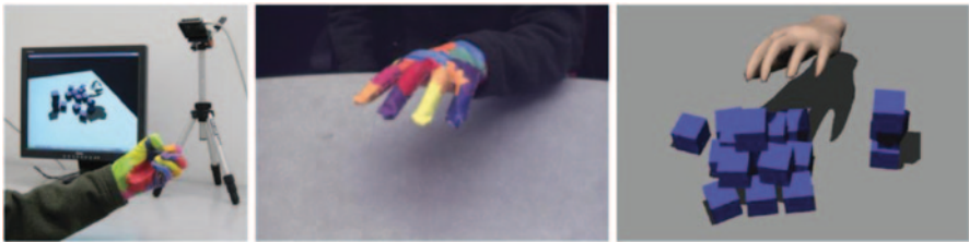
Fig. 2.12 A colored glove system for virtual reality applications. (Courtesy of [18])
