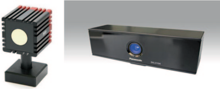
Fig. 3.33 Swiss Ranger 4000 by Mesa Imaging
