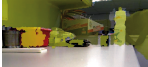
Fig. 3.42 Color Camera view with depth information fused using Kinect
