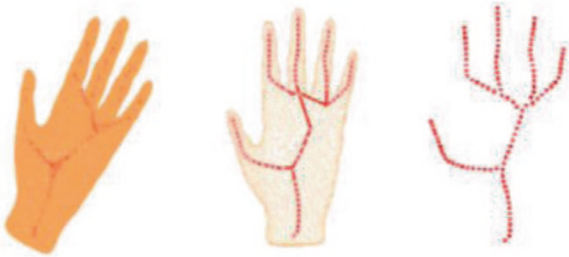
Fig. 3.29 Key points achieved from Laplacian-based contraction and index-based compaction. (Courtesy of [64])
