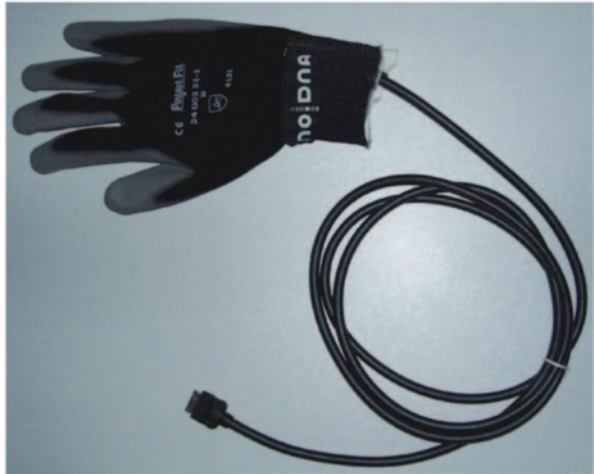
Fig. 2.7 X-IST Data Glove. [12]
