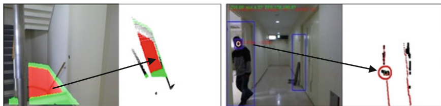
Fig. 8.2 Two samples of navigation map. ( left ) Red region denotes negative obstacle region while green region represent ground plane. ( right ) Human detection and tracking with the personal space assigned (red circle)
