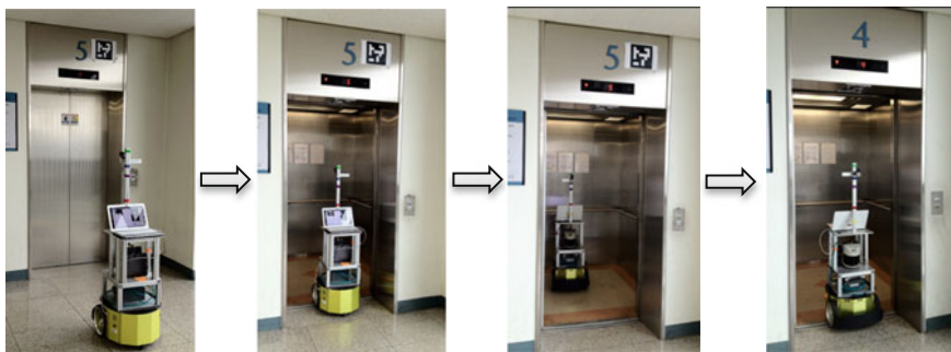
Fig. 11.7 Process of elevator riding: First , door state recognition. Second , floor number and direction classification. Third , get in the elevator and turn toward door. Finally get off the elevator after floor confirming
