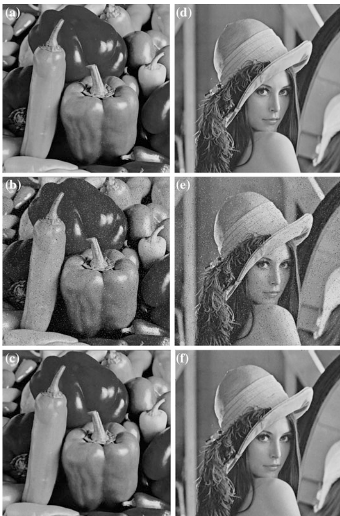
Fig. 17.6 a Original image ( Peppers ). b Received image ( Peppers-before filtering ). c Received image ( Peppers-after filtering ). d Original image ( Lena ). e Received image ( Lena-before filtering ). f Received image ( Lena-after filtering )
