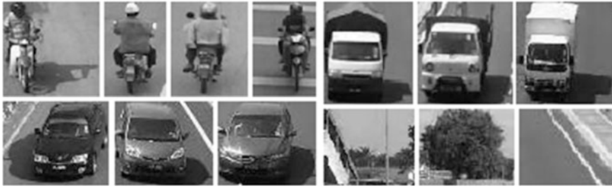
Fig. 26.1 Examples of images used in classification (ViBe’s output images for three different vehicles’ classes and manually segmented background images): from top left motorcycle, lorry, car and background
