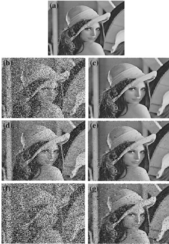
Fig. 27.2 a Lena original image; b 10 % noise image c restored image of (b); d 30 % noise image; e restored image of (d); f 50 % noise image g restored image of (f)
