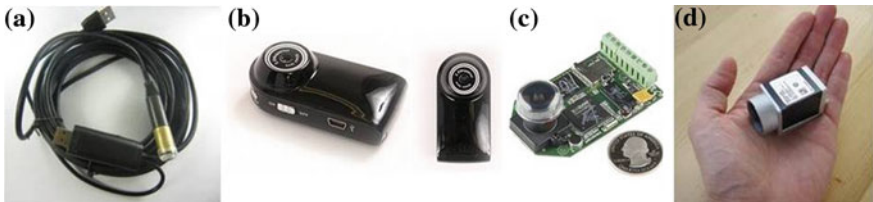
Fig. 59.2 Types of digital camera tested. a USB snake camera with LED. b High definition web camera. c High definition digital board level camera. d High definition network camera
