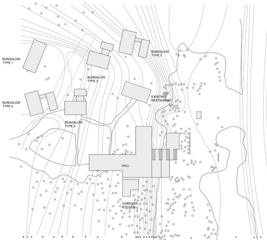
Fig. 5.11 The Port Resolution visitor accommodation facility showing the proposed scheme of bungalows and main hall, with existing site features, levels, trees, grass, sand and water positions recorded during the site survey
