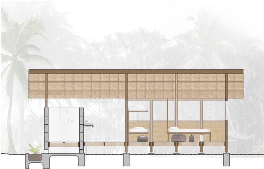
Fig. 5.13 Similar but different: one of the three proposed bungalow types in plan ( above ) and cross section ( below ) showing sleeping quarters separated from ablutions via the use of a breezeway deck: the convenience of proximity is maintained, but privacy, amenity, sanitation, and ease of maintenance are significantly improved
