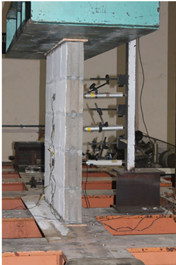
Fig. 3 Experimental set-up for testing of walette
