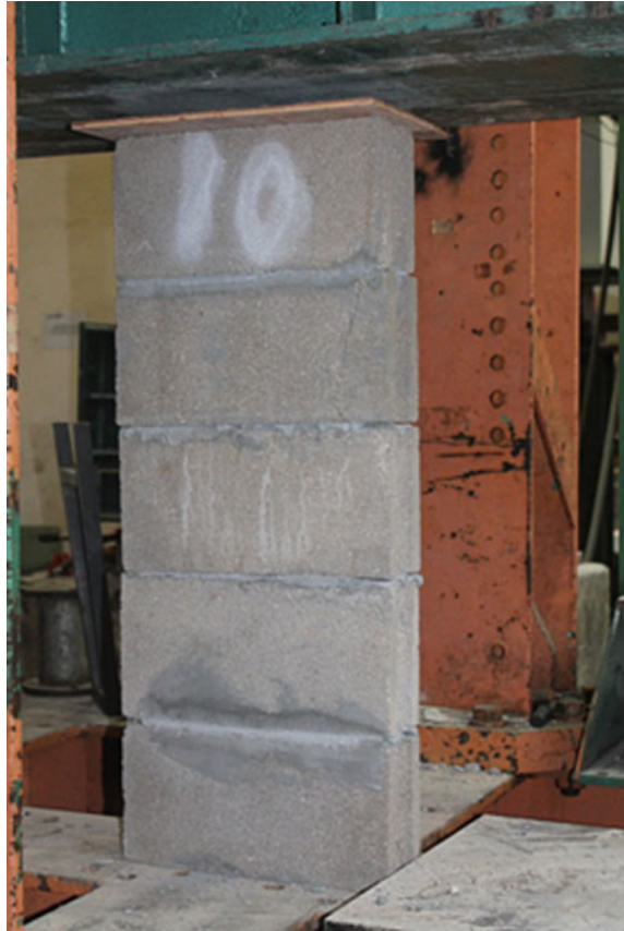
Fig. 4 Experimental set-up for testing of 5-brick prism
