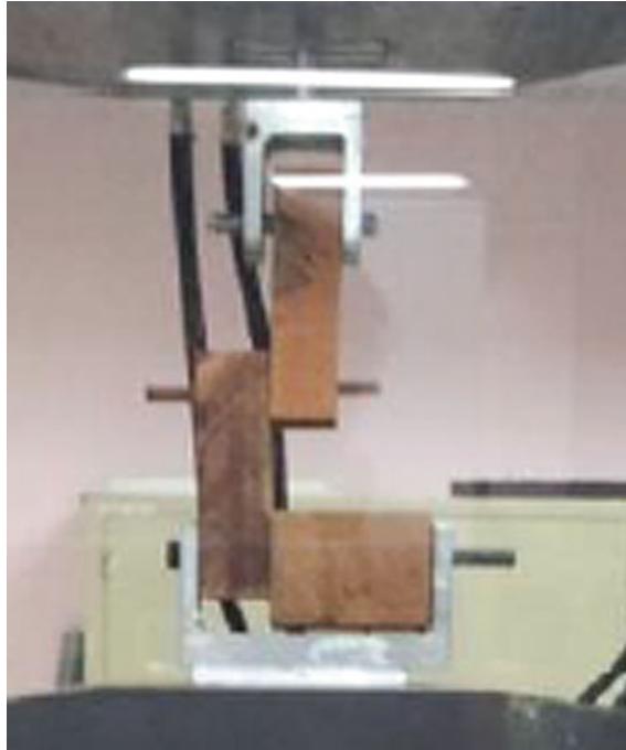
Fig. 6 Typical single shear test setup
