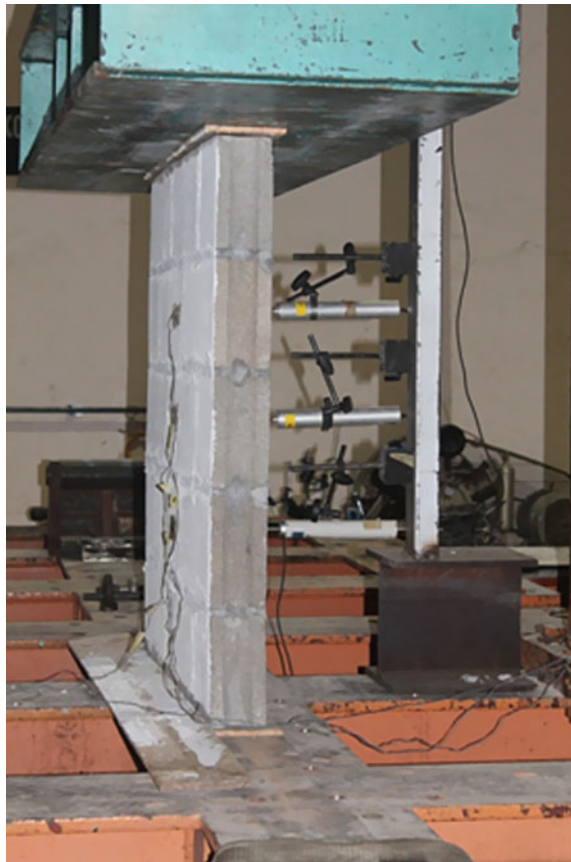
Fig. 3 Experimental set-up for testing of walette
