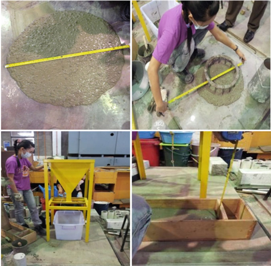
Fig. 3 Testing on fresh concrete properties for SCC
