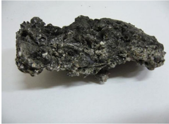
Fig. 2 Porous characteristics of palm oil clinker
