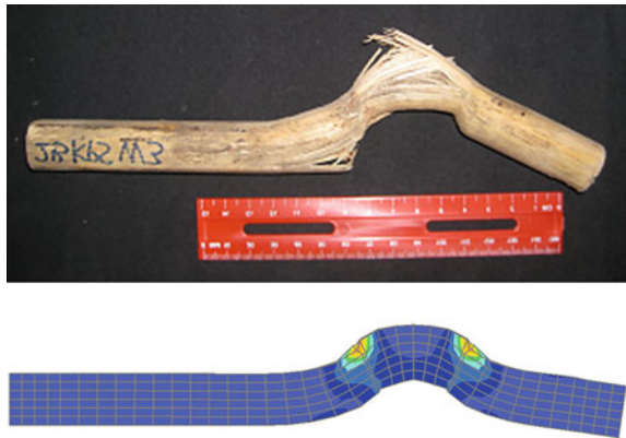
Fig. 4 Total failure of wood dowel in laboratory test (top), deformed shape of dowel in FEM at higher tensile load (bottom)
