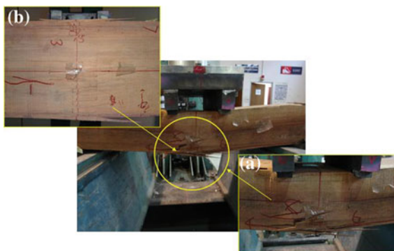
Fig. 5 Solid Kekatong timber railway sleepers showing, a failure started near the tension zone and cracks propagated toward the compression zone; b failure at bottom view of solid timber sleepers
