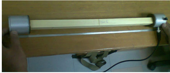
Fig. 1 Test setup for NDT ultrasonic wave test
