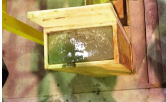
Fig. 4 Observation on segregation of mixture after filling the L-box
