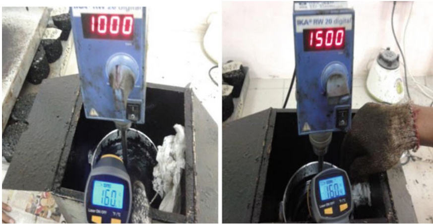
Fig. 1 Mixing process of polymer modified asphalt binder
