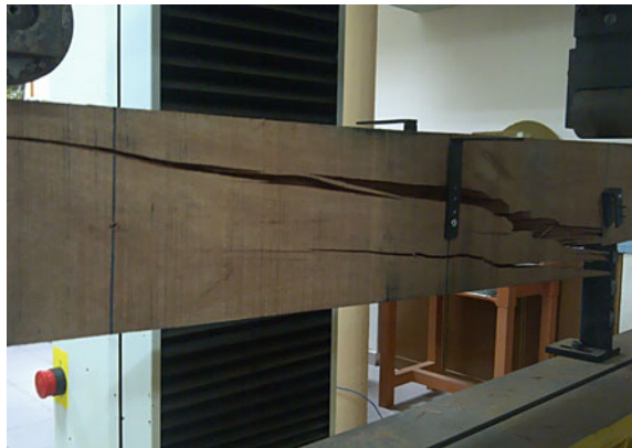
Fig. 7 The crossed-gain failure of structural size test piece was noticeable
