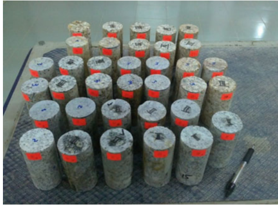
Fig. 1 Samples consist of three grades of weathered granite
