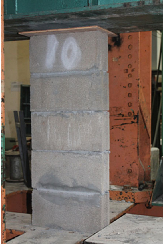
Fig. 4 Experimental set-up for testing of 5-brick prism
