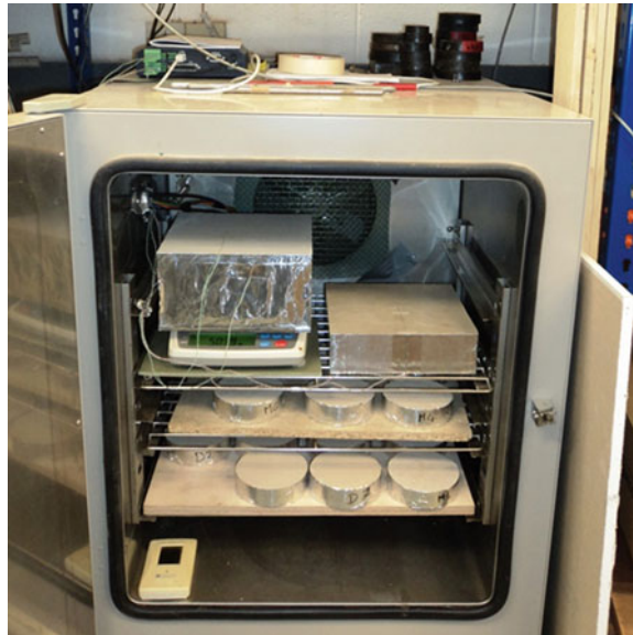
Fig. 1 Climate chamber with electronic balance and samples
