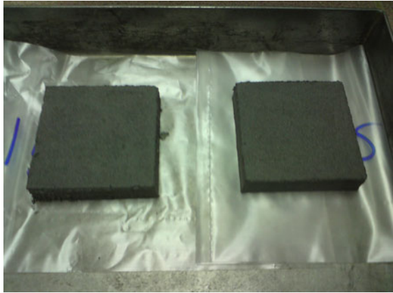
Fig. 1 Preparation of sample for shear box test
