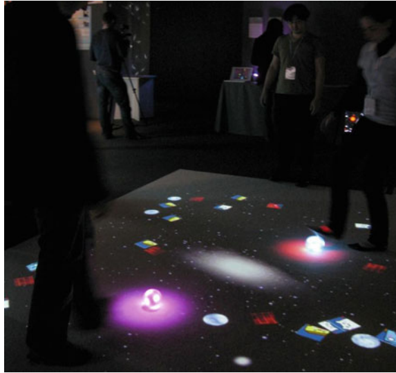
Fig. 10 Collision between the real ball and virtual 3-D objects (a cube and a sphere in virtual space). The “spotlight effect” was applied to the two balls
