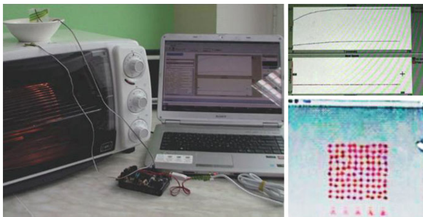
Fig. 19 The melting ice cube model. The toaster oven which was melting the ice and the physical apparatus are on the left . Students created two computer models connected to the sensors: a macroscopic ( top right ) and a microscopic one ( bottom right )
