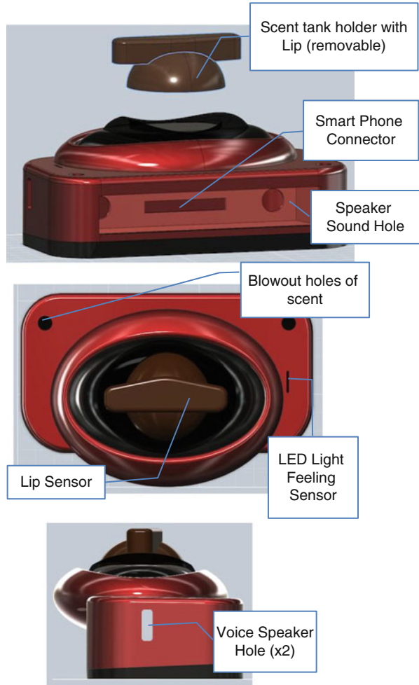
Fig. 8 Key design features of Kissenger
