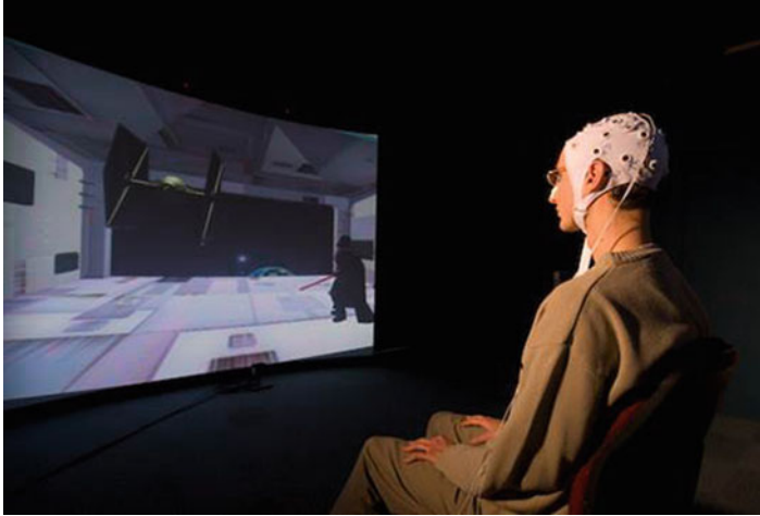
Fig. 1 The “Use-the-force” application. The user had to lift up a virtual spaceship using foot motor imagery (©CNRS Phototèque/Hubert Raguet)
