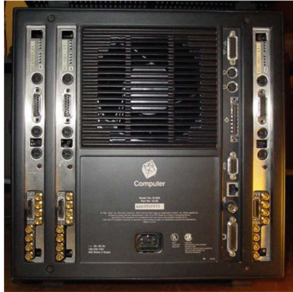
Fig. 13 An IRCAM Signal Processing Workstation (A NeXt Cube workstation with three i860 boards installed) (Photo courtesy of Mr. Jean-Bernard Emond)
