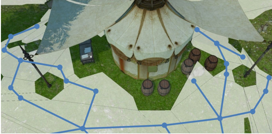
Fig. 14 Navigation meshes and linked graph structure of Final Fantasy XIV (Final Fantasy XIV © 2010–2016 Square Enix Co., Ltd. All Rights Reserved)
