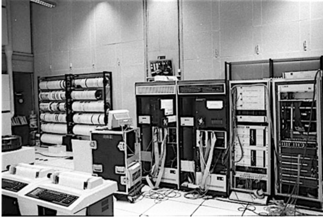
Fig. 11 The IRCAM 4X (the hardware with the cables in the racks in the center) (Photo by Martin Guy, This image is from Wikimedia and licensed under Creative Commons Share-Alike 1.0 License)
