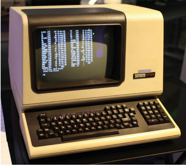
Fig. 5 DEC VT-100 Terminal (Photo by Jason Scott. This image is from Wikimedia and licensed under the Creative Commons BY 2.0 license)
