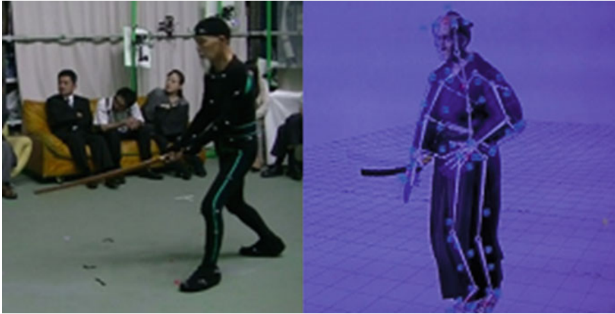
Fig. 12 Performance of the craft of drawing out the sword and CG Samurai drawn with the motion data (Endo 2015)
