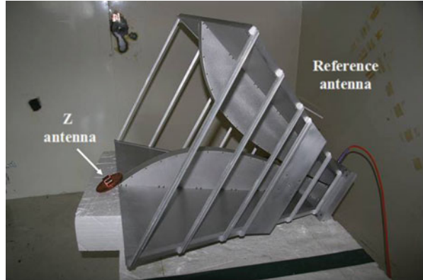
Fig. 8 Physical comparison of the 570 MHz small ground plane Z antenna and the dual-ridged reference horn in the NIST-Boulder reverberation chamber
