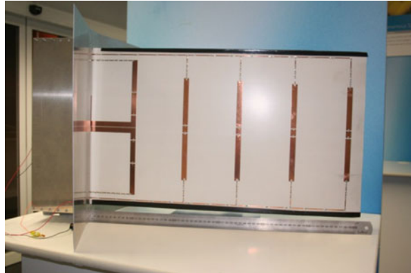
Fig. 2 Photo of the frequency reconfigurable UHF antenna (with a 60 cm long metallic ruler)
