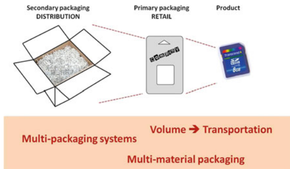
Fig. 1 Examples of packaging designs that increase the environmental burdens of the product: multipackaging systems, volume increase, and multimaterial packaging
