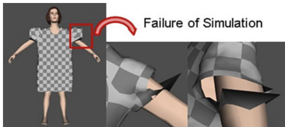
Fig. 7 Example of bad prepositioning which leads to failure of simulation
