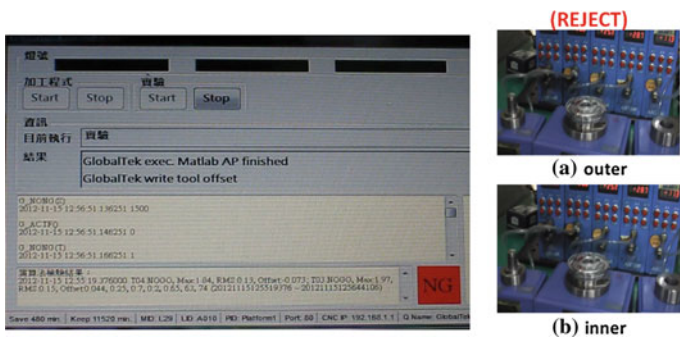
Fig. 4 Result of ‘No-Go’ case from online quality inspection system
