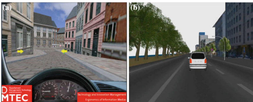
Fig. 1 a Template scene of the attention test—two arrows were simultaneously presented and participants were asked to report whether the orientations of two arrows were the same b Template scene of the motion detection test—a front car with different speed settings was presented and participants were asked to report whether the speed of the front car was faster or slower than his/her own speed
