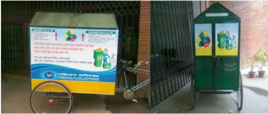
Fig. 4 Three chambered waste collection vans for separate collection
