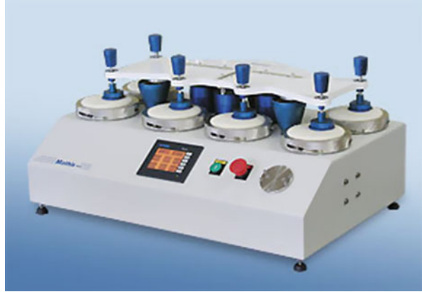
Fig. 24 Abrasion resistance test equipment (Reproduced with permission from Mathis et al. [46]. Copyright 2014)
