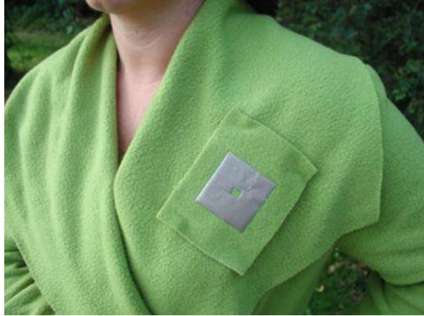
Fig. 1 Textile microstrip patch antenna. Antenna patch and ground plane patterned in Zelt electro-textile. Fleece material used as antenna substrate
