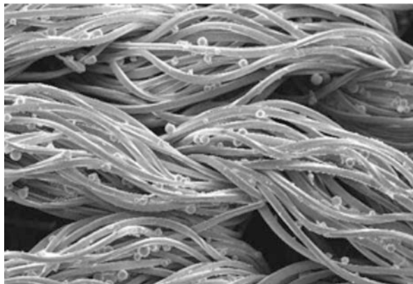
Fig. 9 Fabrics coated with phase change materials by printing. (Outlast Technologies LLC, http://www.outlast.com/en/applications/ . Reprint with permission)
