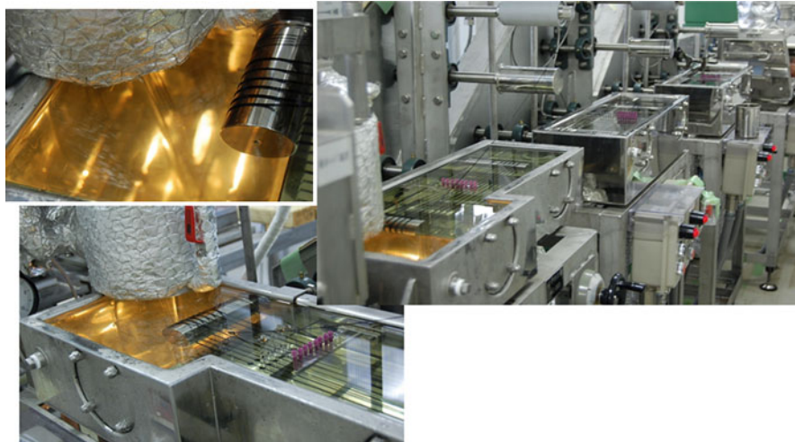
Fig. 2 Photographs of custom-built wet-spinning apparatus for PEDOT:PSS/PVA blended multifilament fiber (© 2014 WILEY-VCH Verlag GmbH & Co. KGaA, Weinheim)
