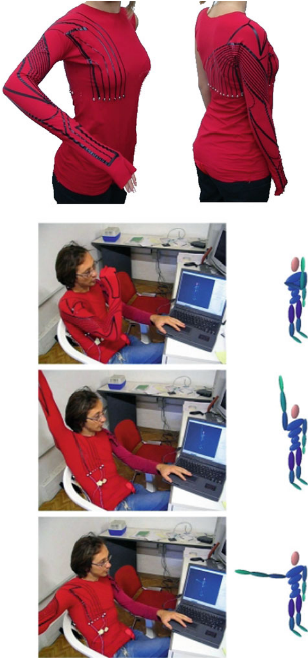
Fig. 17 The UKLG prototype and posture recognition trials performed by the user and represented by the avatar (Reproduced with permission from Ref. [4])
