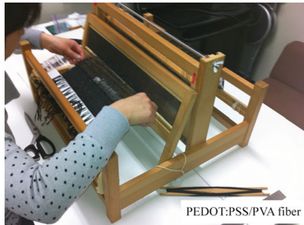
Fig. 5 Photograph of weaving apparatus for the preparation of textile electrodes using PEDOT: PSS/PVA blended fibers (© 2014 WILEY-VCH Verlag GmbH & Co. KGaA, Weinheim)
