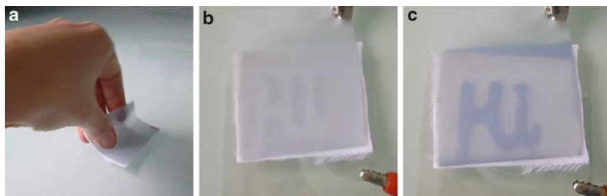
Fig. 22 F-ECD containing PEDOT:PSS in its (a) oxidized and (b) neutral (reduced) states [51]
