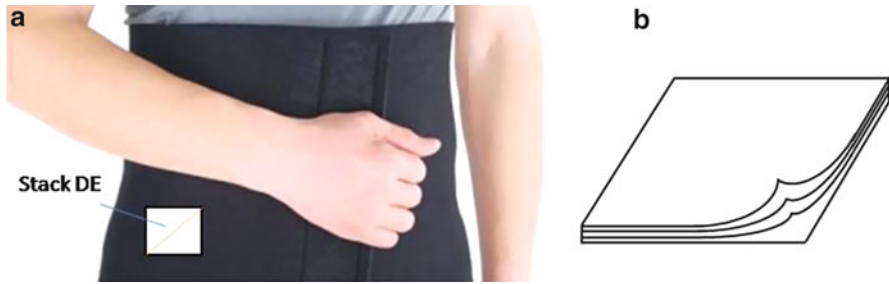
Fig. 13 Illustration of a stack DE-driven slimming belt (a) and stack DE actuator (b)
