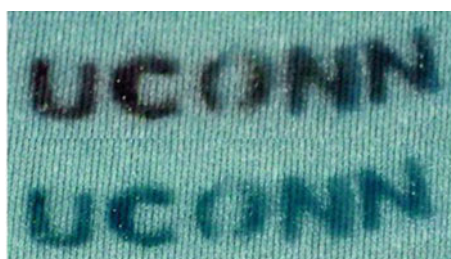
Fig. 24 Stencil-patterned solid-state fabric ECD in its neutral ( top ) and oxidized ( bottom ) state (Image reprinted from Invernale et al. (2010) ACS Applied Materials and Interfaces 2:296, with permission of the American Chemical Society) [53]
