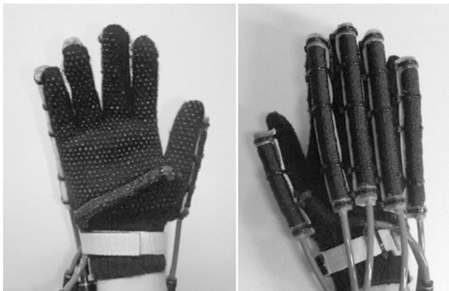
Fig. 12 Wearable power assist devices for rehabilitation using pneumatic artificial rubber muscle (With permission from Elsevier)
