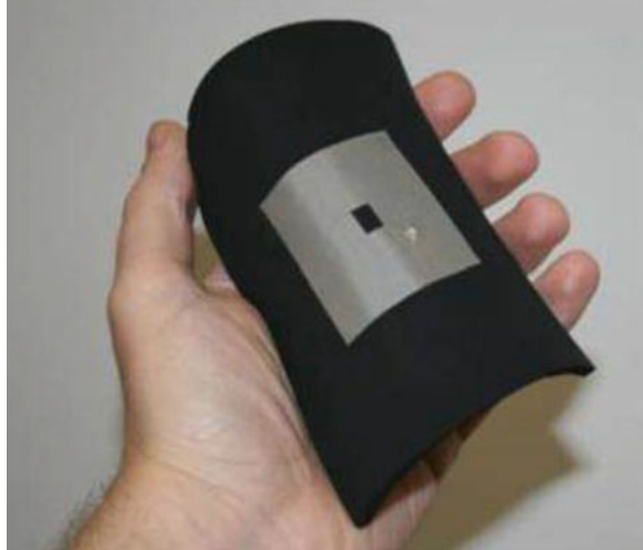
Fig. 3 Flexible circularly polarized textile microstrip antenna. Copper-nickel-plated nylon used for antenna patch and ground plane. Protective foam applied as antenna substrate
