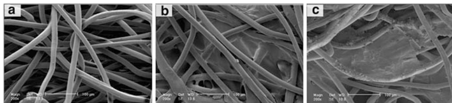
Fig. 16 SEM micrographs of unmodified nonwoven PP fabrics (a), PNIPAAm-g-PP (grafting yield = 15.7 %) (b), and PNIPAAm/β-CD-g-PP (grafting yield = 6.92 %) (c) (Reprinted from Amiri et al. [59] with permission from SAGE Publications)
