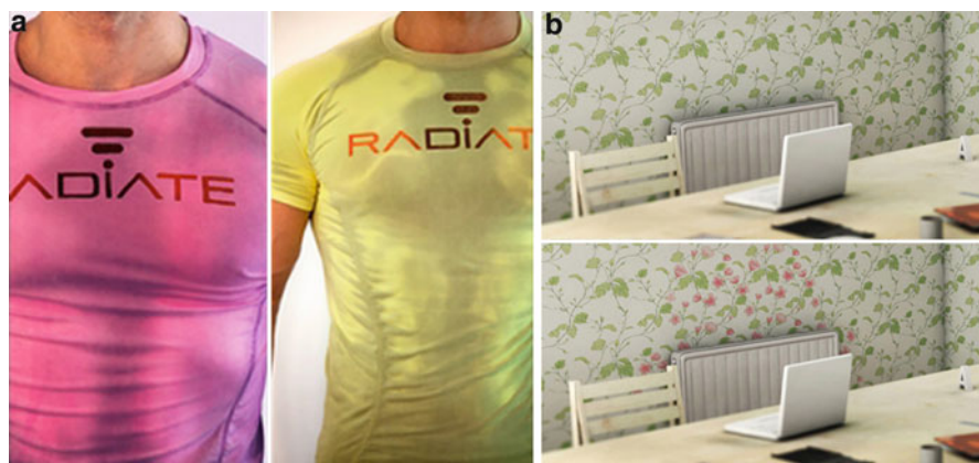
Fig. 3 Thermochromic textiles: (a) Radiate Athletics' heat-sensitive sportswear (Image reprinted with the permission of Radiate Athletics http://www.radiateathletics.com/ ) [12] and (b) Shi Yuan's blossoming wallpaper (Image reprinted from Meunier et al. (2011) Indian Journal of Fibre & Textile Research 36:429) [49])
