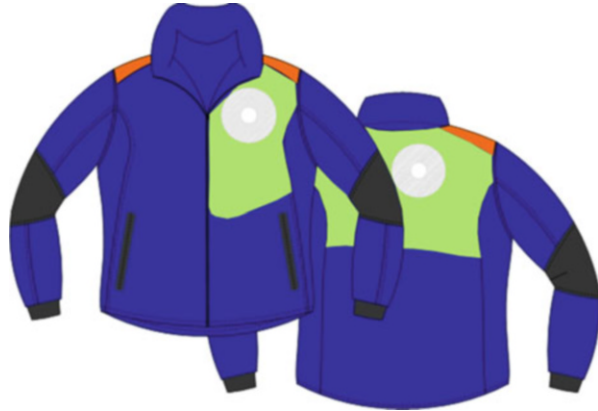
Fig. 5 Wearable rectenna placement on a technical garment (Taken from our Ref. [10] (Conference EuCAP 2011))
