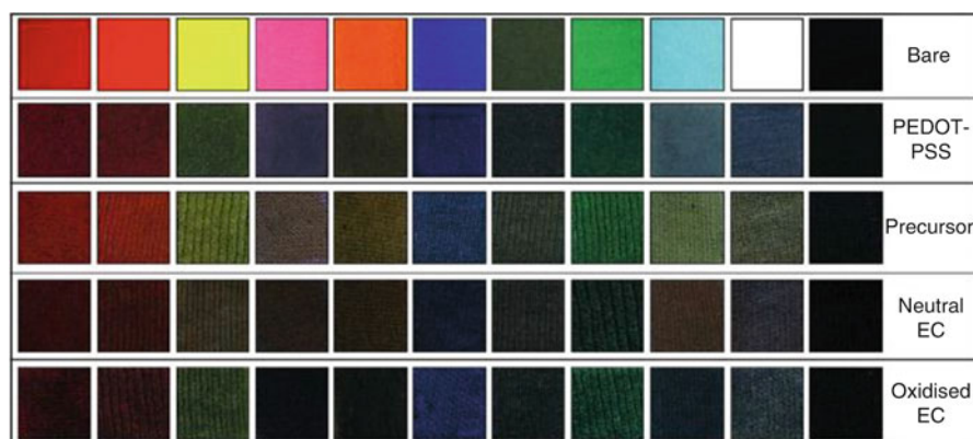
Fig. 25 The effects of PEDOT:PSS in the (a) precursor, (b) oxidized, and (c) neutral states, on the color of dyed fabrics (Image reprinted from Invernale et al. (2011) Coloration Technology 127:167) [55]
