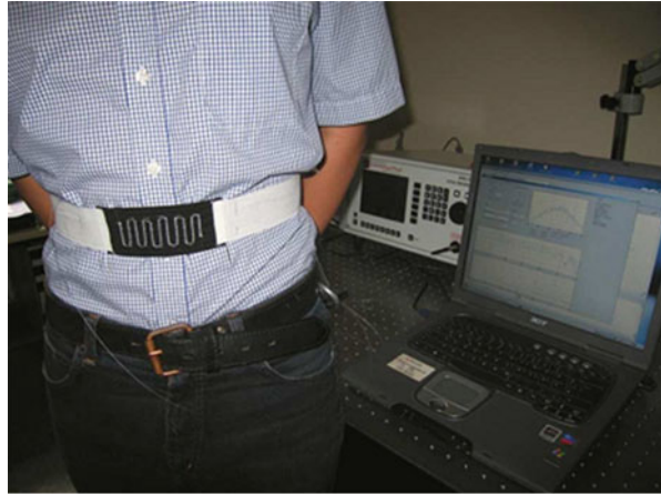
Fig. 8 Abdominal respiratory of an adult monitored and recorded by POF OTDR (Copyright 2002, IEEE, License Number: 3554190358248)
