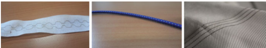
Fig. 4 Examples of electro-conductive tracks made by Elasta and VDS Weaving (UGent)
