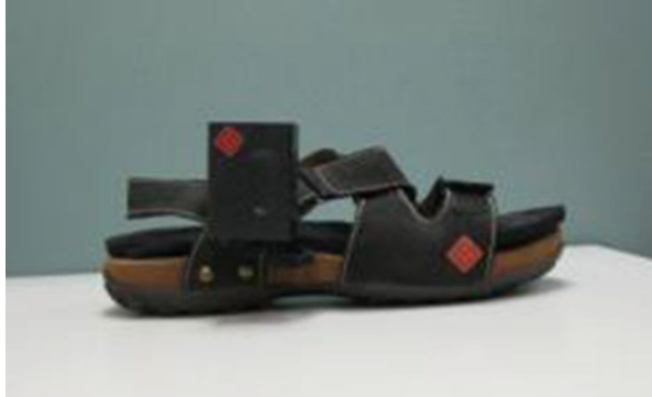
Fig. 11 Prototype of the in-shoe plantar pressure measurement system (Reproduced with permission [27], Copyright 2010, IEEE)
