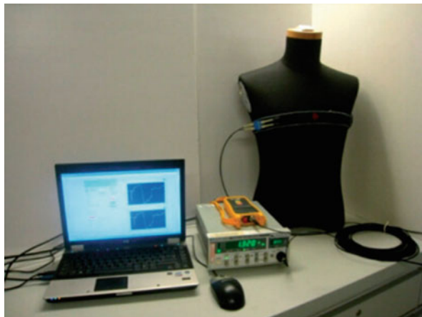
Fig. 9 Human respiration monitoring system based on four-loop fabric POF sensor [48] (Copyright 2014, SAGE)
