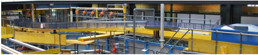
Fig. 4 Overview of the physical model with Lake Geneva tank on the right , Veytaux 1 powerhouse in the background, and Veytaux 2 powerhouse on the far left
