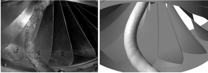
Fig. 2 Comparison of the vortex rope shape observed at the model test and numerically simulated at part load and high head
