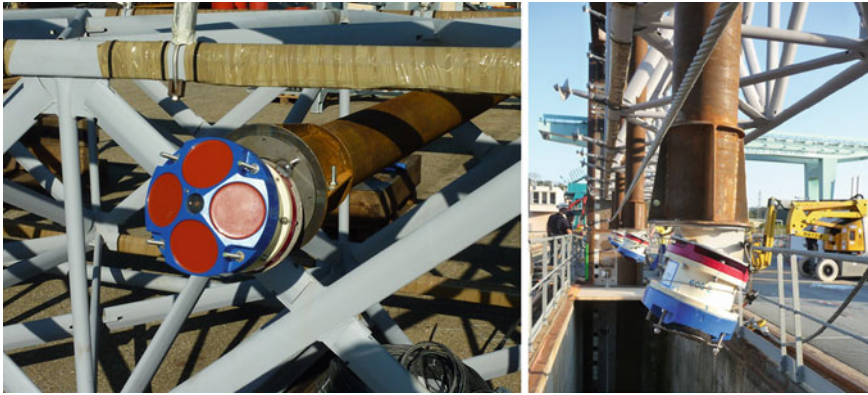
Fig. 6 Workhorse Rio Grande ADCP placed on vertical position on measurement frame
