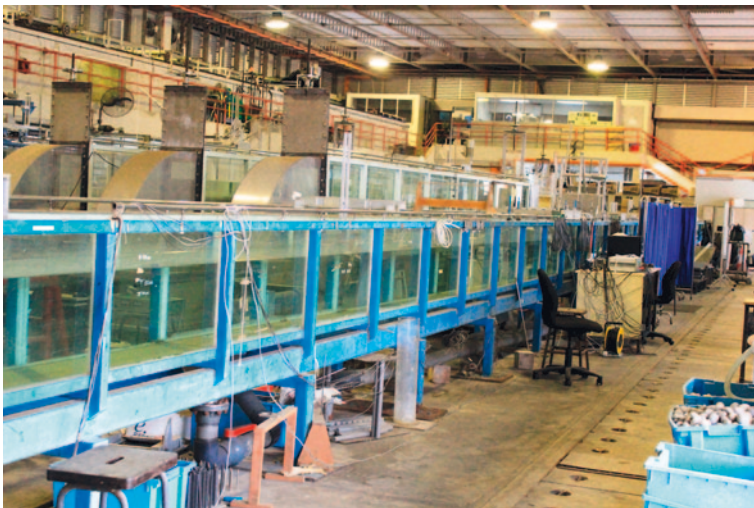
Fig. 6.2 The 36 m-long wave tank at Nanyang Technological University (NTU) in Singapore. The facility is designed for laboratory studies of wave behaviour and wave interaction with coastlines of various configurations (Photo courtesy of Mr. Shawn Sim, NTU Department of Civil Engineering and the Earth Observatory of Singapore)
