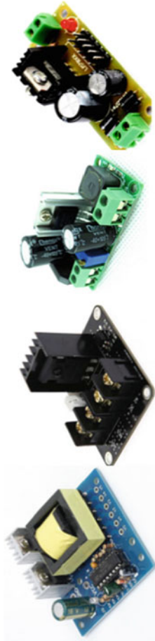
Fig. 1 Examples of low cost heatsinks applied to commercially available small electronic power converters
