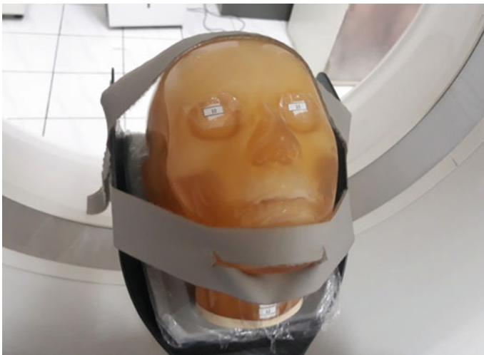
Fig. 2 Placement of TLDs in the right and left eyes and on the thyroid
