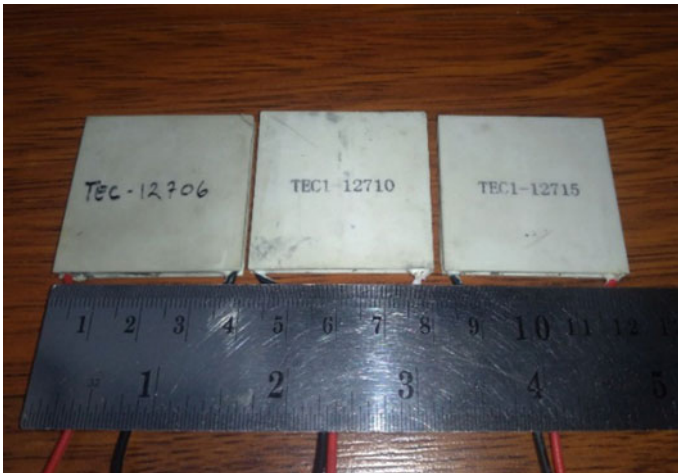
Fig. 2 Selected thermoelectric generator module, TEC1-12706, TEC1-12710, TEC1-12715
