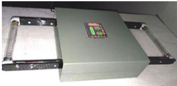
Fig. 3 The infant incubator sterilizer with two ultraviolet germicidal lamps on both sides
