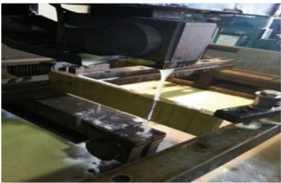
Fig. 9 Calibration block during and after wire cut process
