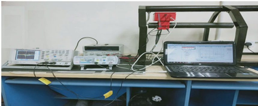
Fig. 2 Piezo Lamb Wave testing inspection system (PZ-LW)
