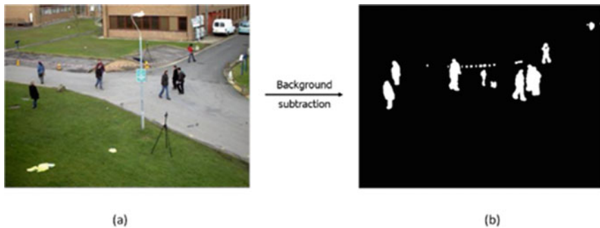
Fig. 2 Motion detection: a original image and b moving parts
